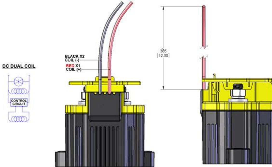
WIRE SPEC: SILICONE, 22AWG, -40C-150C, UL: VW-1
