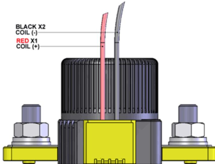
WIRE SPEC: SILICONE, 22AWG, -40C-150C, UL: VW-1
