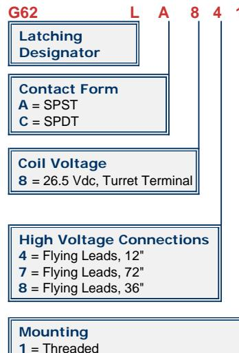
\*Order the relay with the part number as shown. The latching "L" designator and the coil voltage will not appear in the P/N on the relay but will be indicated on the label that is on the base of the relay. Observe coil polarity.
