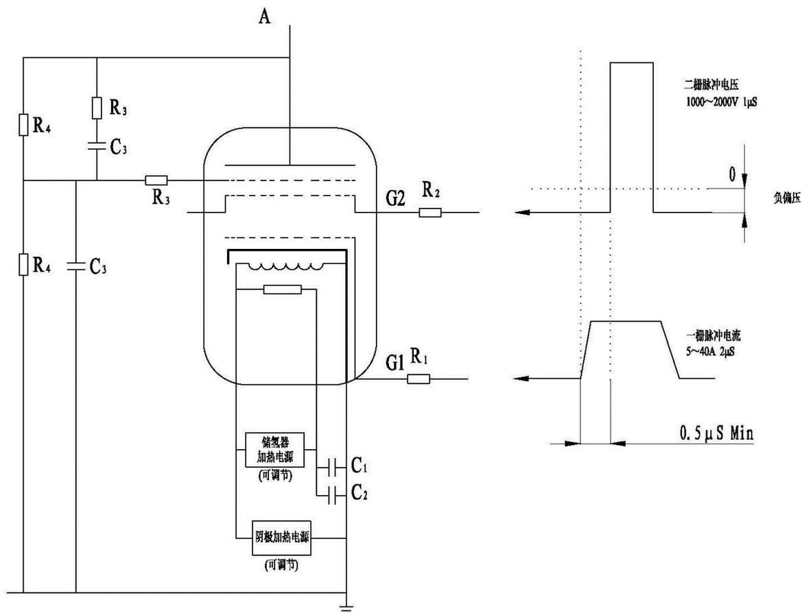
R1 Grid 1 series resistor. 12W vitreous enameled wire wound is recommended, its impedance matches with the trigger's circuit impedance.
