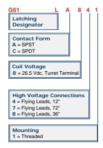
Order the relay with the part number as shown. The latching "L" designator and the coil voltage will not appear in the P/N on the relay but will be indicated on the label that is on the base of the relay. Observe coil polarity.
