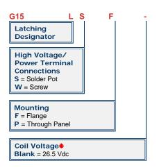
\*Order the relay with the part number as shown. The latching "L" designator and the coil voltage will not appear in the P/N on the relay but will be indicated on the label that is on the base of the relay. Observe coil polarity.
